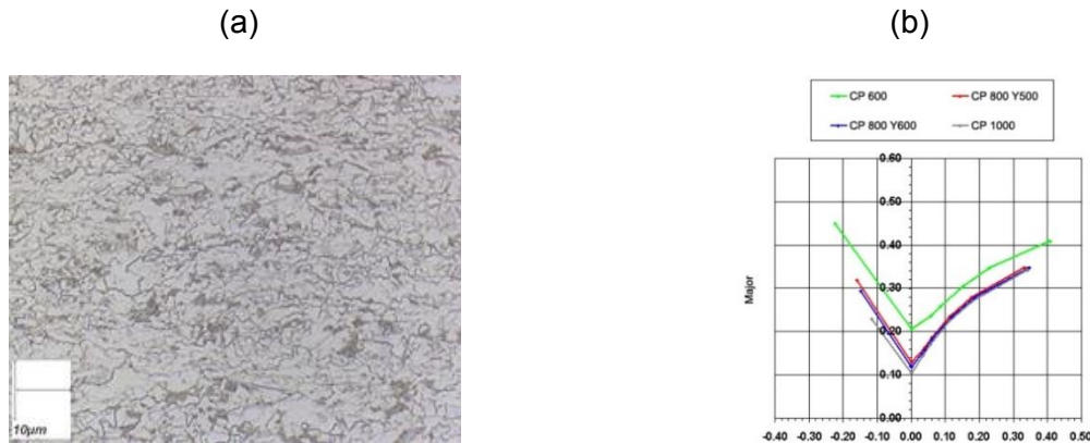
Fig. 19.(a) CP800 steel microstructures, b-) FLDs of various CP steels [ArcelorMittal].
