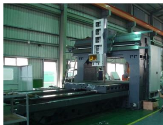
Fig. 2 Bridge type machine tool. (Courtesy of Vision Wide Tech Co., Ltd.)
