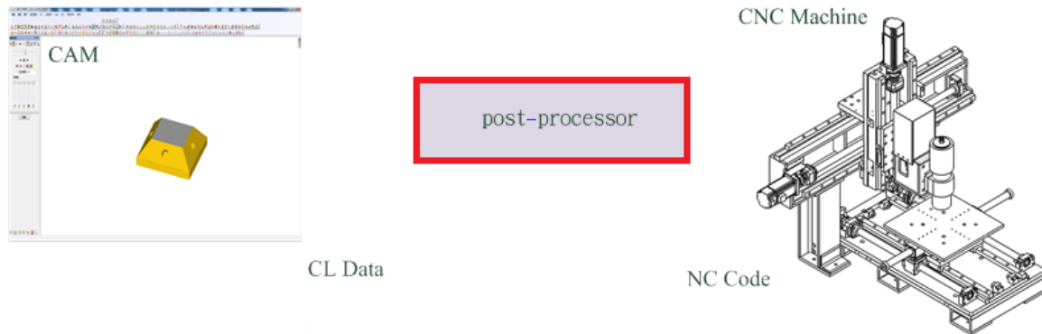
Fig. 6 Relationship between CAM, postprocessor and CNC.
