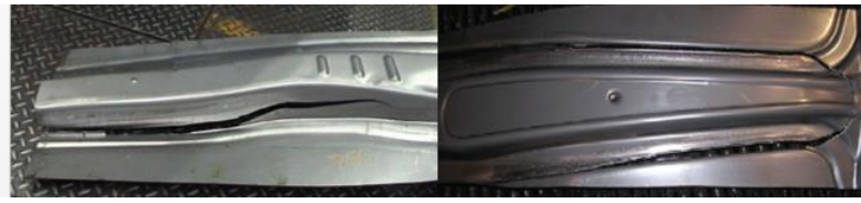
(b) DP790 Underbody structural part and DP980 B-pillar inner [Chen, et al., 2005]
