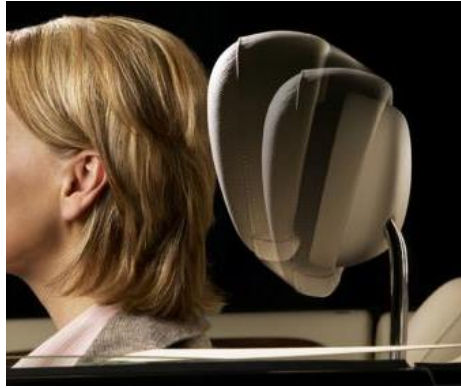
Figure 5: The movement of the NECK-PRO relative to the occupant's head (Daimler, n.d.).
