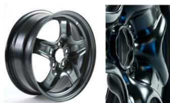
Fig. 13. (a) Bumper from DP 1180, (b) Wheel web from hot rolled DP 600, (c) B-pillar reinforcement from DP 980 [ArcelorMittal].
