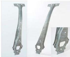
Fig. 15(a) B-pillar reinforcement in TRIP 780, (b) Bumper cross member in TRIP 780 [ArcelorMittal].
