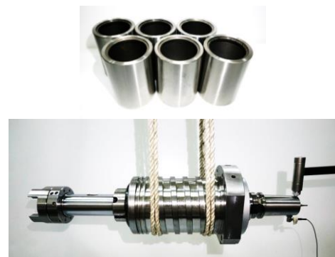
Fig.2 Bearing spacers and configuration of vibration test.
