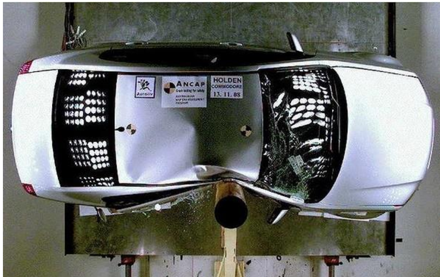
Figure 1. Pole side impact test in line with FMVSS 214 (adapted from www.ancap.com )
